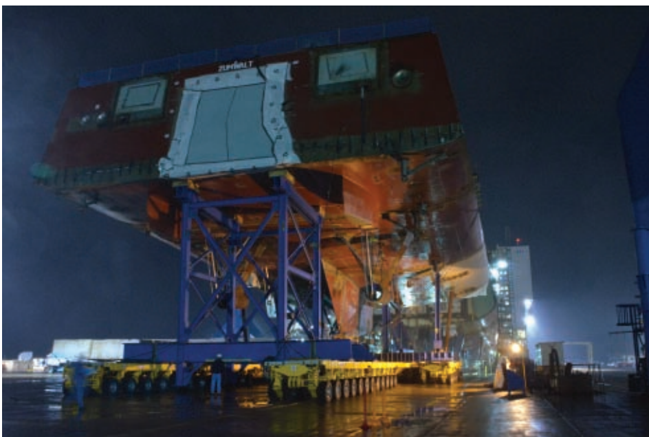
Ultra 3200 moving into place on the Land Level. Photo by P. Cummings
