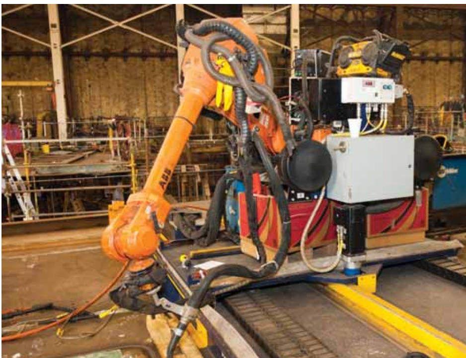
The portable ABB Robotic Welding machine.
